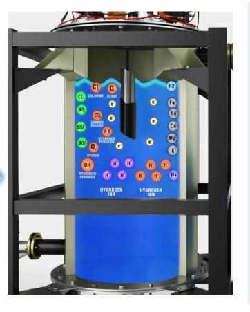
Electricity is When passed through the anode and cathode. The dissolved Ion will precipitation start due to polarity of charges. Chlorine and Other oxidizers are due generated reaction. The Scale which causes damage of fils and poor HEX will be ACCUMILATED on the Cathode.
